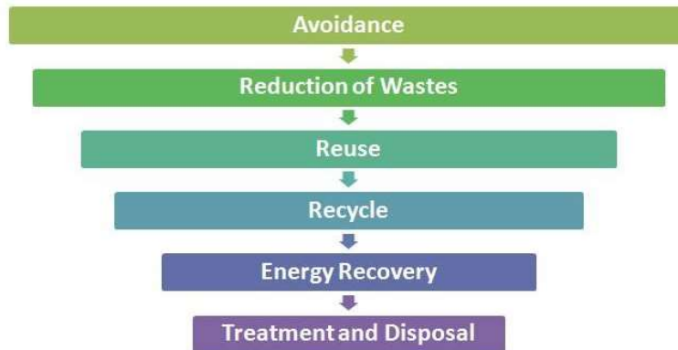
Fig. 1. Waste Hierarchy list in order of preference from the most favorable (top) to the least (bottom).
